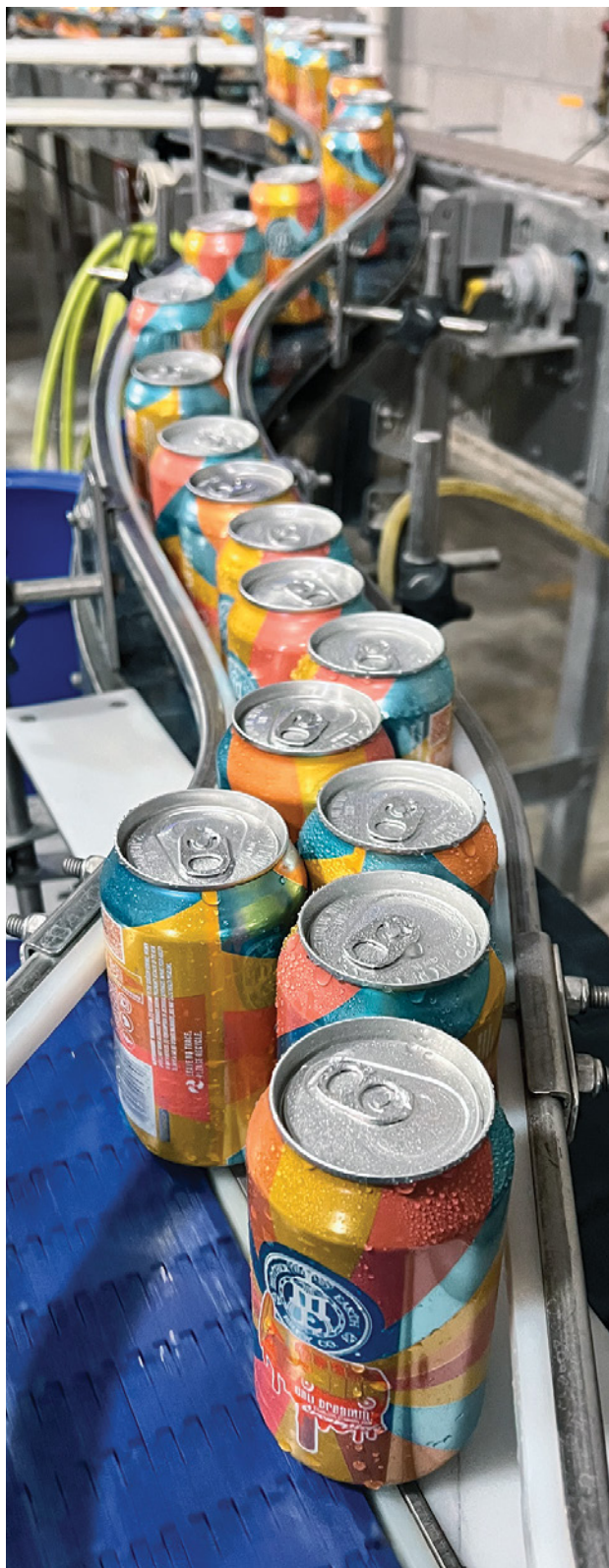
Cans on their way into a PakTech can carrier applicator 120/180. The applicator can be configured for a six-pack or four-pack. From there, a long infeed conveyor brings cans to the Econocorp cartoner.
