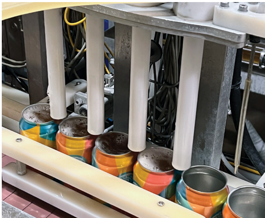
The cans run through two separate Wild Goose WGC 250 canning lines, where cans are rinsed and sanitized by two twist rinsers, filled, and sealed.
