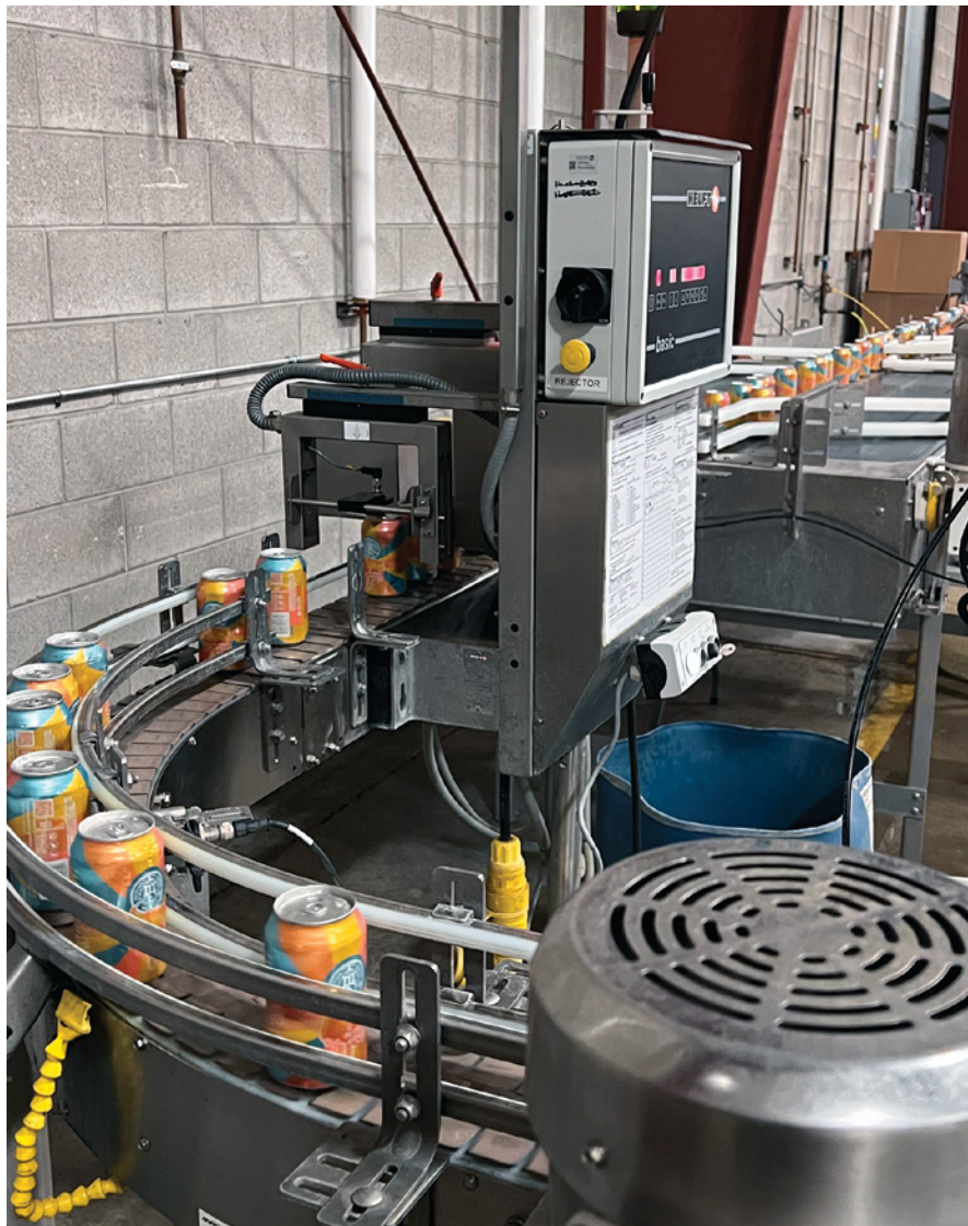
Custom conveyance brings the two Wild Goose lines together and sends cans through a Heuft Basic low fill/low pressure detector.
