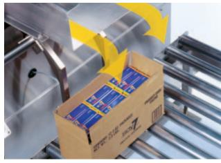
$\label{lowered} \mbox{Loaded case is pneumatically lowered for discharge}$
