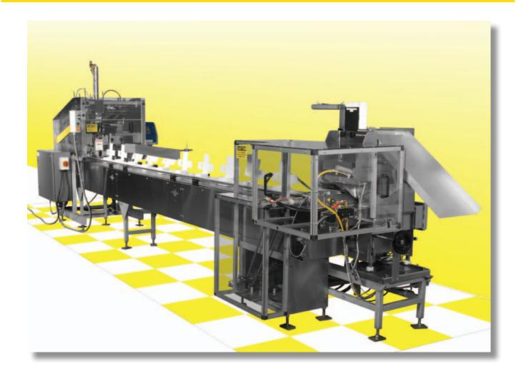
A completely automatic system for forming, conveying, closing and sealing top loaded cartons.
