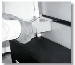
1. Operator presents one end of a carton in position over the glue pot and starts the cycle via a foot pedal.
