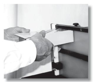
2. Carton is then manually lifted against a squaring device on the compression panel and hot melt seals the carton flaps.
