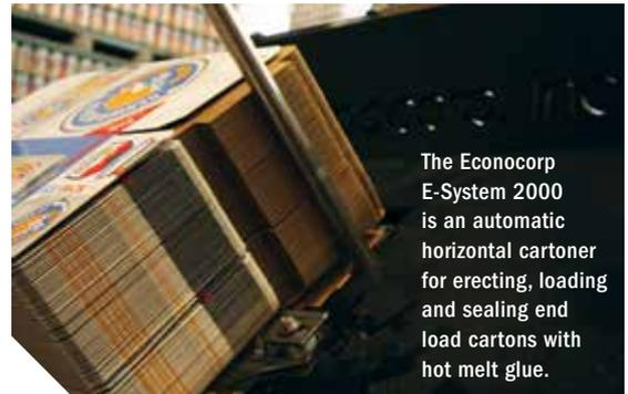
The Econocorp E-System 2000 is an automatic horizontal cartoner for erecting, loading and sealing end load cartons with hot melt glue.
